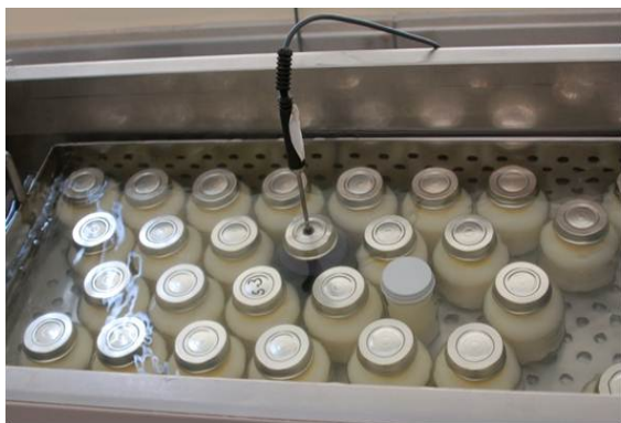
Figure 2: Milk is pasteurized in a water bath > 62.5^{\circ}\text{C} for 30 min
